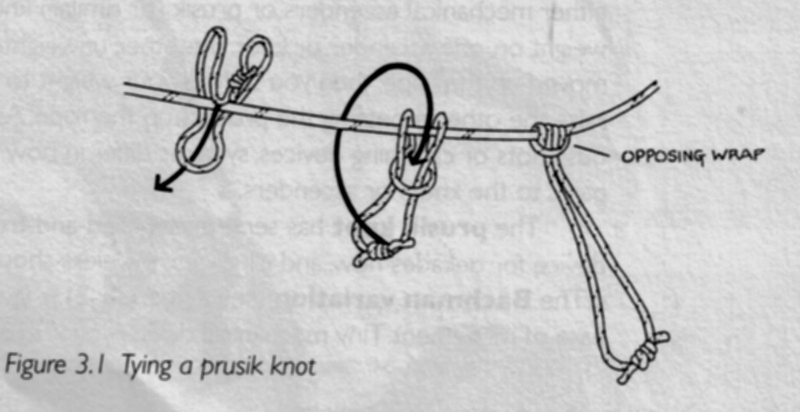
prusiks because its very supple sheath grabs extremely well. However, be aware that this softer sheath wears faster than the stiffer but tougher perlon. The new nylon-sheathed, 5.5mm Spectra cord is a suitable, prusik material that's essentially as strong as a climbing rope, although even the softer weaves are a bit stiffer than perlon. Kevlar cord should never be used for a prusik because it's quite stiff and its fibers readily break down with repeated flexing.
